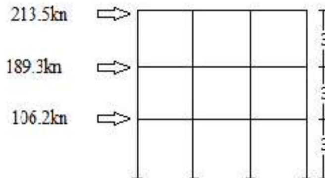
Fig 3. distribution of lateral load according to ASCE 7-10
