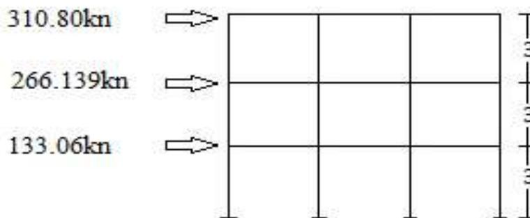
Fig.2. Distribution of lateral load according to EC8
