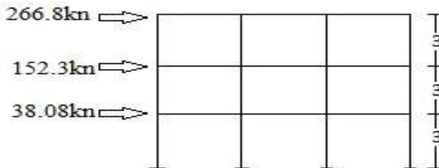
Fig no. 1. Lateral load on each storey
