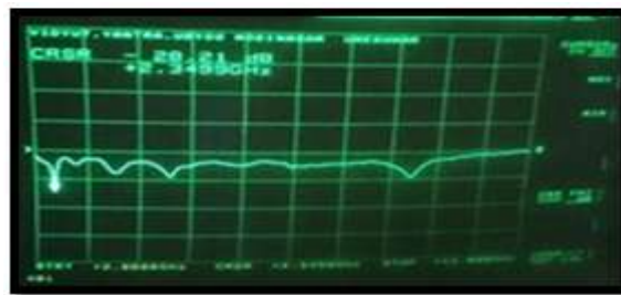
Figure 1.7: Graph plot at 2.34 GHz of proposed fabricated antenna
