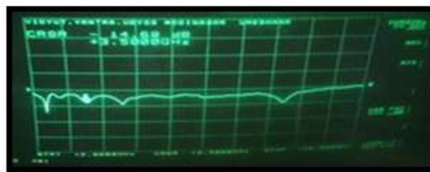
Figure 1.9: Graph plot at 3.5 GHz of proposed fabricated antenna
