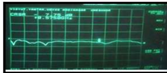
Figure 1.11: Graph plot at 8.57 GHz of proposed fabricated antenna
