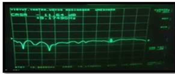
Figure 1.12: Graph plot at 9.17 GHz of proposed fabricated antenna
