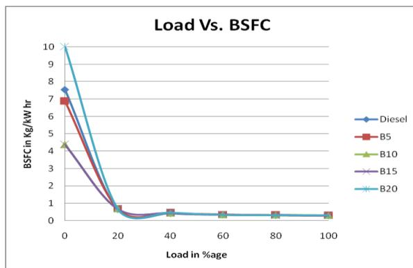
Fig -7: Variation of the BSFC with Load
