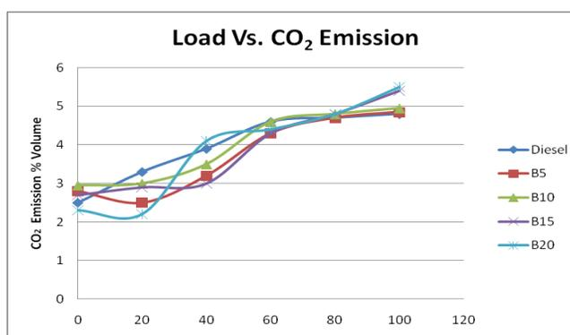
Fig -14: Variation of the Emission of CO<sub>2</sub> with Load
