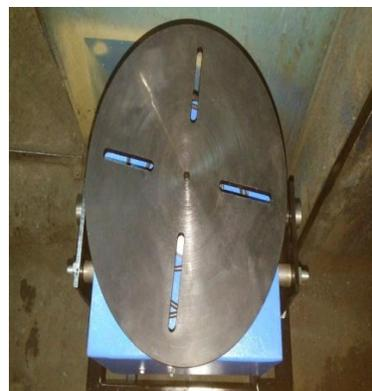
Fig 6.2 Indexing Plate
