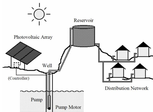
Fig.5 - Village water supply flow diagram
