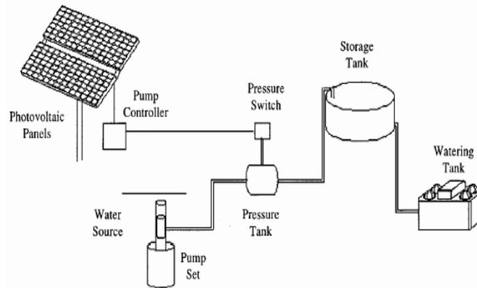
Fig.3 - Direct coupled solar pumping system
