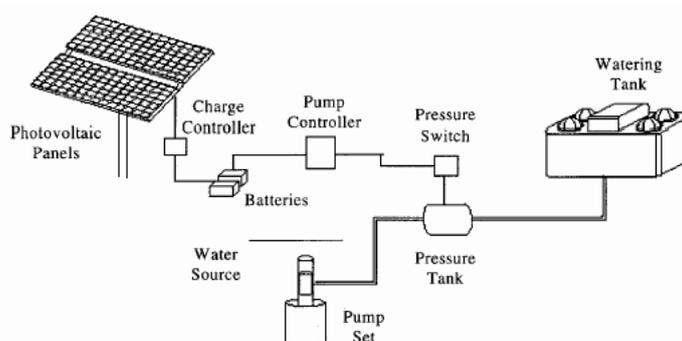
Fig.2 - Battery-coupled solar water pumping system
