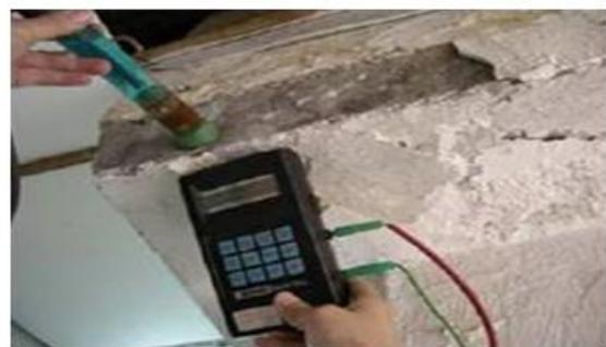
Half-Cell Potential Test of Slab
