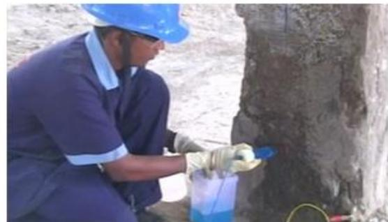
Half-Cell Potential Test of Column
