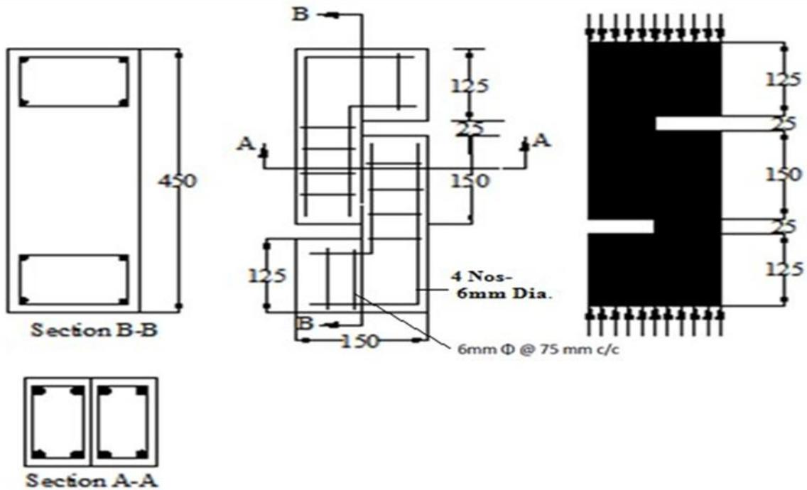
**Reinforcement in Push-off for shear Specimen**
