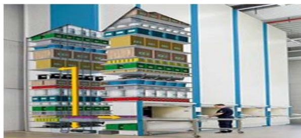
Figure 1 STO lift machine used in industry<sup>[12]</sup>
