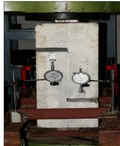
**Fig.2: Laboratory set up for the Push-off Specimen**
