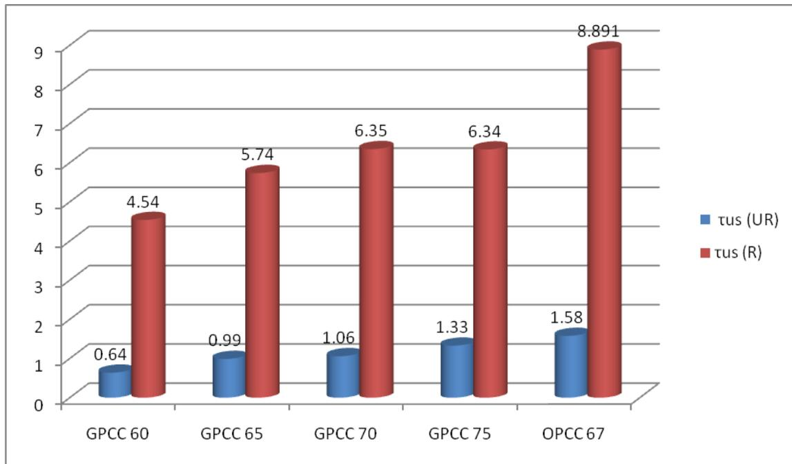
**Bar Chart No.2:- Depicting Ult. Shear Strength of GPCC (Both Reinforced & Un-Reinforced) w.r.t. Total Aggregate Contents from Table no.10.i.e.inferity of GPCC w.r.t.O.P.C for Total Aggregates Percentages.**
