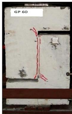
**Figure 3: Crack pattern in reinforced push-off Specimen GPCC60**
