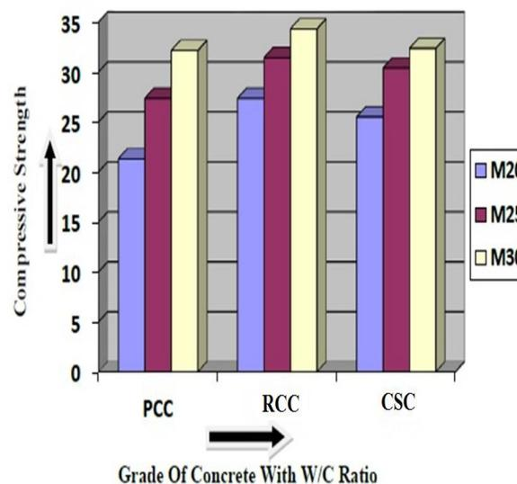
**Graph 1. Compressive Test result of coconut shell concrete**
