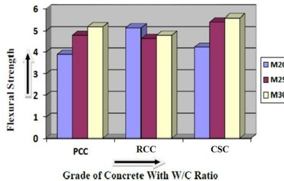
**Graph 3. Flexural Test result of coconut shell concrete**
