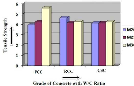
**Graph 2. Tensile Test result of coconut shell concrete**
