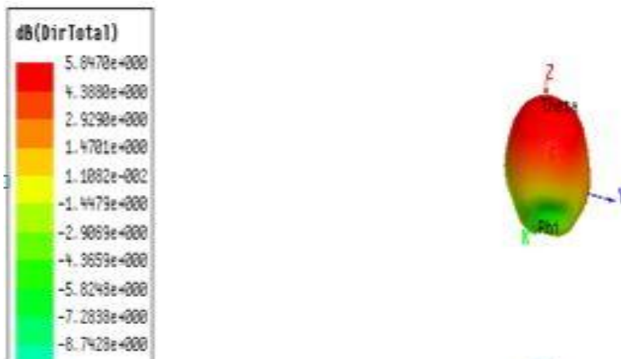
FIG.5: Directivity of proposed antenna
