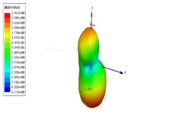
Any antenna is said to have 100% efficiency if the obtained gain and directivity are equal. The gain and directivity of the proposed antenna are nearly equal.
