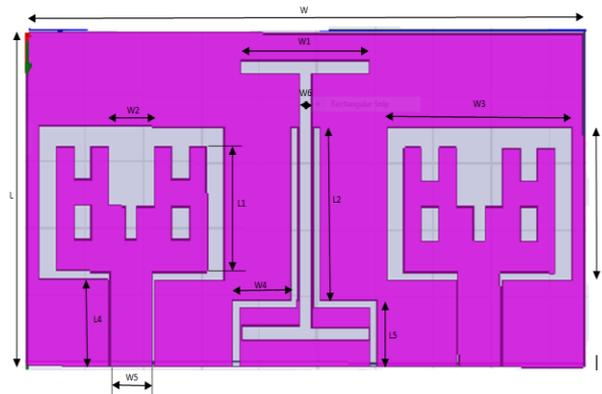
**Fig.3 Design of the Antenna with Dimensions**
