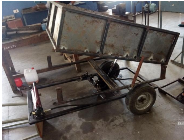
Fig: Modern Three Way Dumping Trolley Layout
