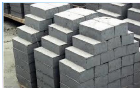
Figure 6: Bricks manufactured from fly ash
