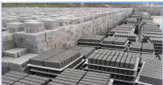
Figure 6: Bricks manufactured from fly ash
