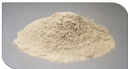
Figure 2: Fly ash (Cement like powder) and particles of fly ash
