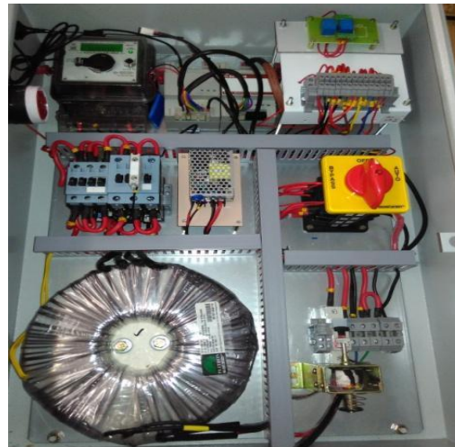
Fig.2 Single phase of street light controller
